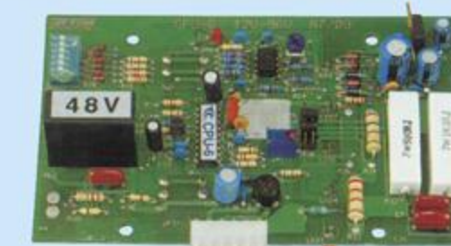
A PCB with supervise functions gives a safe charging
